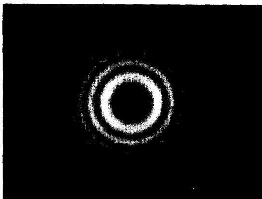
Figure 8 : Interference pattern obtained with the two-parallel foils arrangement
