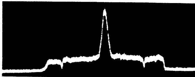
Fig. 7 : Vertical beam profile. The pedestal is due to the electrons from the rest gas. Indentations in the pedestal are the \pm 20 mm fiducial marks.
