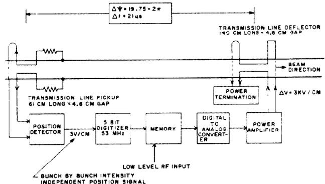
Fig. 2. Block diagram of the digital feedback vertical damper.
