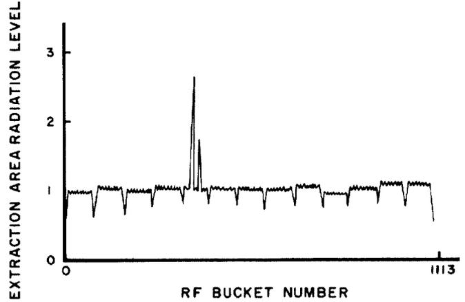
Fig. 1. A radiation monitor near the extraction channel is observed on an oscilloscope triggered at the revolution frequency. The gaps occur between each of the 13 batches injected by the booster synchrotron. A few bunches have blown up and show large losses.
