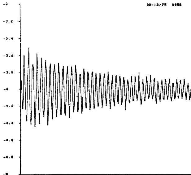
Figure 8. Booster radial betatron oscillation digitized by the Nicolet.
