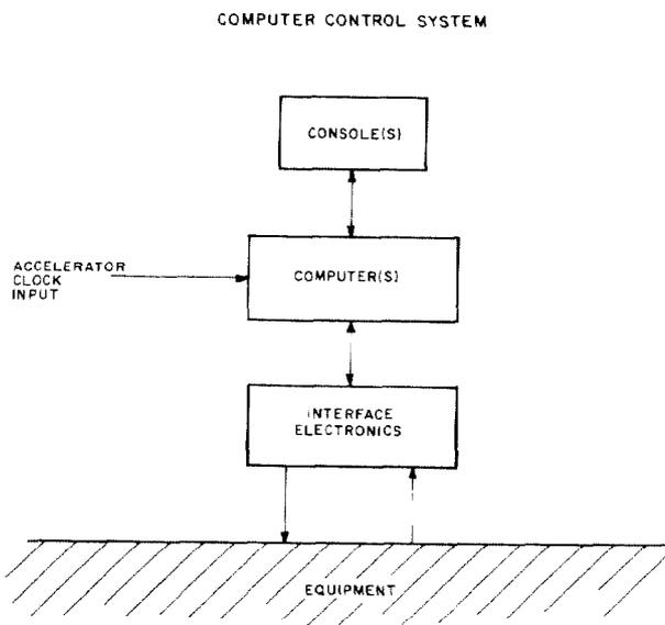
Figure 1. Simplified Computer Control System
