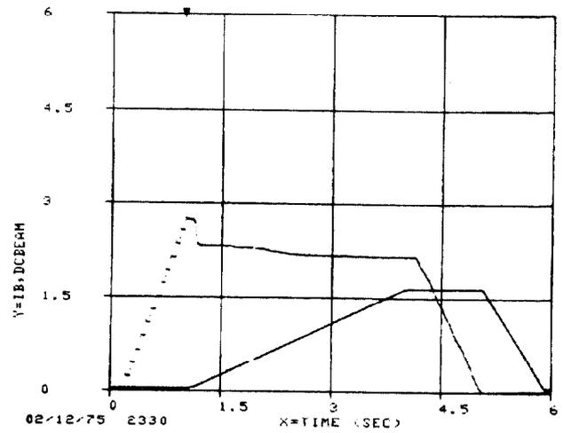
Figure 4. Fast time plot of the main magnet ramp and accelerator beam.
