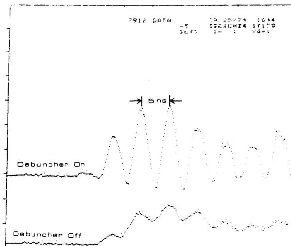
Figure 9. First turn booster beam showing the effects of the debuncher on the 200 MHz structure.
