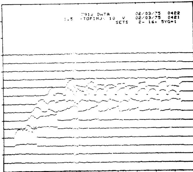
Figure 12. Digitized wire scanner data 5  $\mu$ sec/division.
