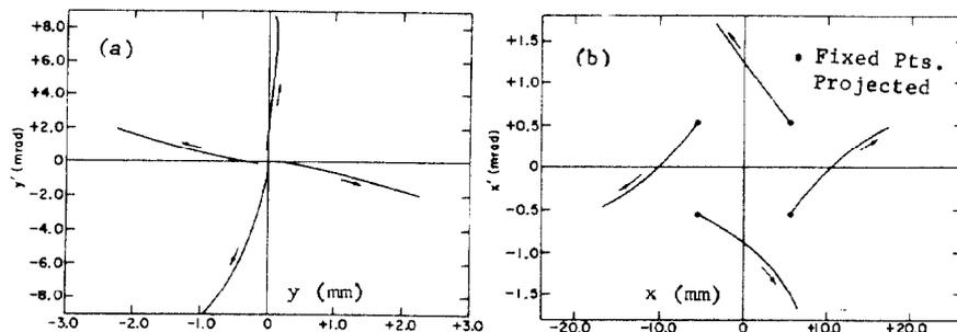
Fig. 5. 4th order sextupole resonance. Unstable trajectory. (a) Vertical projection, (b) Horizontal projection. Initial conditions  $[x=+5.5\text{mm}, x'=+0.55\text{mrad}, y=+0.25\text{mm}, y'=0.0]$ .
