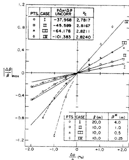
Fig. 2.  $|\Delta\beta/\beta|_{\text{max}}$  vs  $\Delta p/p$ . Chromaticity corrected in normal cells. The period phase advance,  $\nu_c \sim 3/4$  integer. Straight lines are theoretical estimates. Numerical results from SYNCH.
