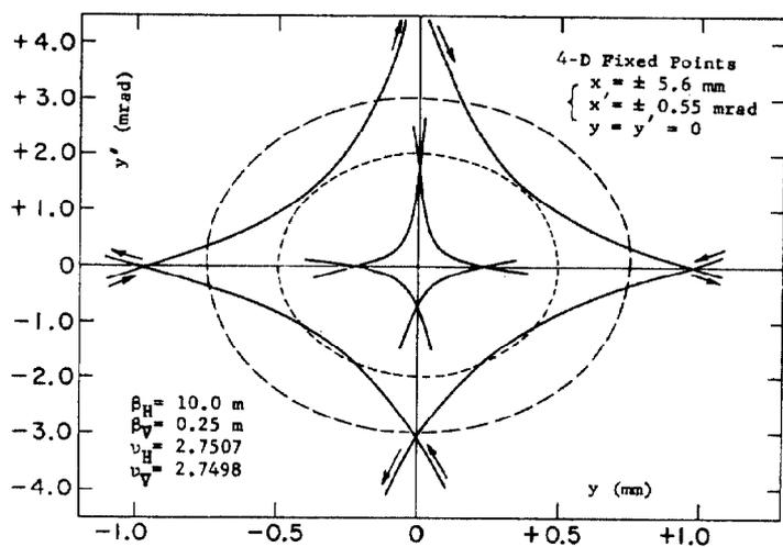
Fig. 4. Phase space topology near 4th order fixed point. Vertical projection. 4th order sextupole resonance. Elliptical plots are non-resonant trajectories. Corresponding motion in  $[x, x']$  projection remains near fixed point. The apparent "trajectory crossings" are not fixed points, but are artifacts of the 2-dimensional projection.
