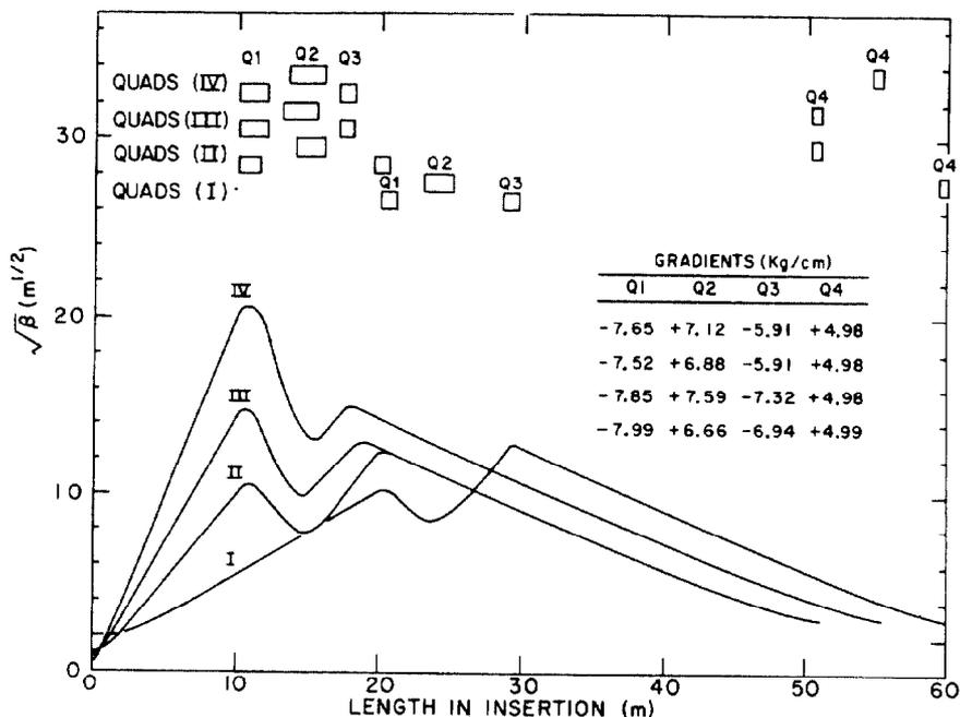
Fig. 1.  $\beta$ -function for low- $\beta$  matched insertions.  $\beta_{\text{cell}} = 9.0$  m. Q4 is a lattice cell quadrupole.
