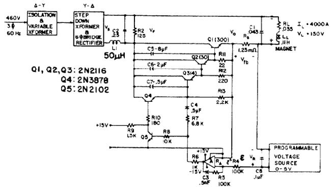
Fig. 1. Circuit Schematic Current Regulated Power Supply.
