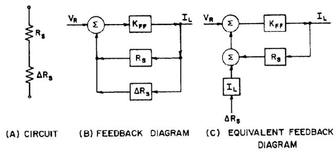
Fig. 6. Effect of Variation in Current Sensor.
