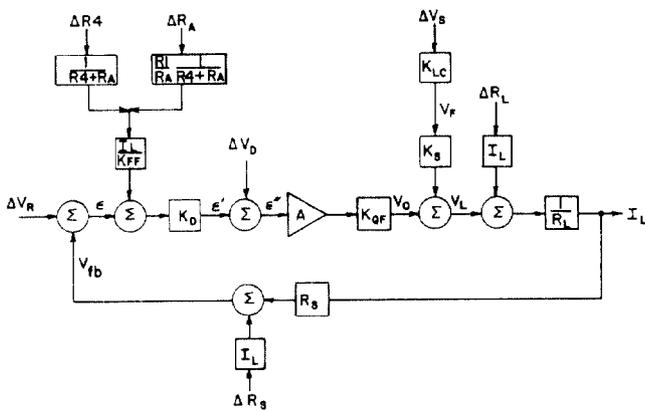
Fig. 5. Feedback System Disturbances on Output Current.
