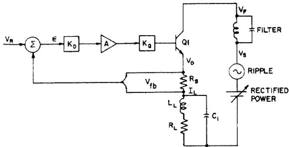
Fig. 4. Hybrid Block Diagram Power Supply as an Emitter Follower.
