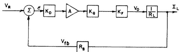
Fig. 3. Simplified Block Diagram Feedback System (dc).
