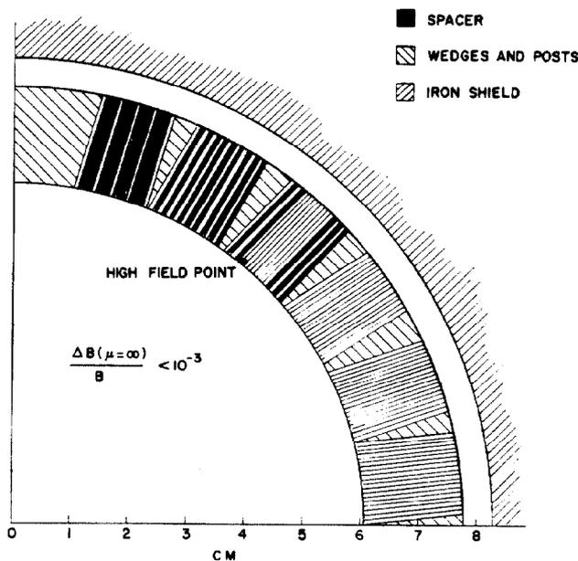
Fig. 1. The turns distribution for the full-scale ISA magnet.
