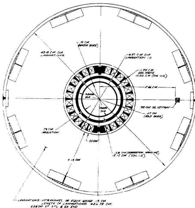
Fig. 2. The overall cross section of the 12-cm dipole (shield and coils).
