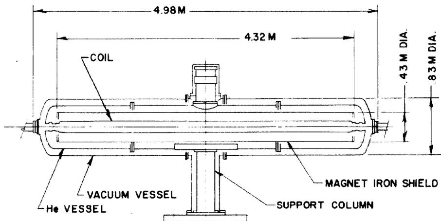
Fig. 5. The ISA size 4.25-meter magnet and dewar assembly.
