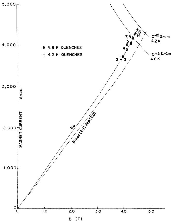
Fig. 6. This is a graph (I vs B) in which the load line of ISA IV is plotted with quench points indicated. The curves for the  $10^{-12} \Omega\text{-cm}$  equivalent resistivity for the wire used in the magnet are included as well.
