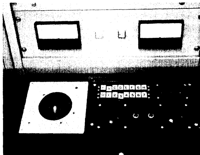
Fig 2: Close-up of operator station input hardware. Meters and two interrupts are above; trackball/GO button at lower left; push-button matrix, digit switches, two shaft encoders and two levers at lower right.
