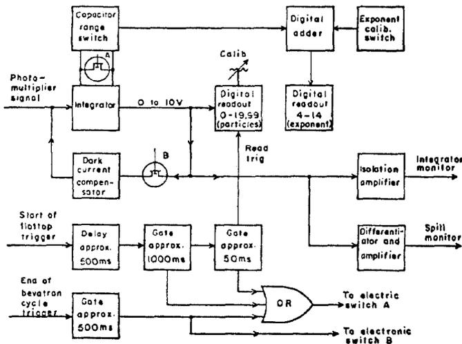
Calibration is accomplished at the low intensity end by reducing the beam level until the scaler P.M. signal is linear. The HV on the integrating P.M. is then adjusted until the digital voltmeter readout corresponds to the scaler read out. The integrator output now reads particles per pulse. The output from the integrator will now be linear until the P.M. saturates, either current saturation in the final stages or saturation at the photocathode.
