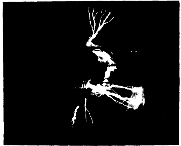
Fig. 4 High voltage sparks from terminal to ground at 9 MV photographed from the end of the accelerator through special windows.
