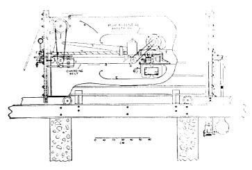
Fig. 1. First electrostatic accelerator insulated by high pressure gas, 1934.
