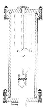
Fig. 3. First successful getter-ion pump. Titanium wire, T, is evaporated from the graphite crucible, C, to provide gettering action. Ion pumping is accomplished by a grid ionizer, G, utilizing electrons from filament, F.
