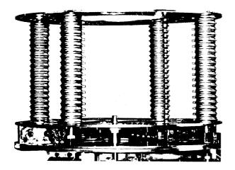
Fig. 7. Column module composed of four identical and interchangeable support posts bolted to metal coupling and transition sections. Each module with accelerating tube (not shown) carries a rating of one million volts.
