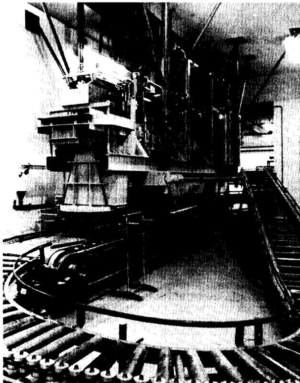
Fig. 10. 10 MeV Linac for Irradiation Processing.
