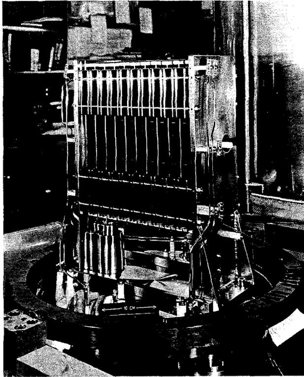
Fig. 6. Model of inflector magnet.
