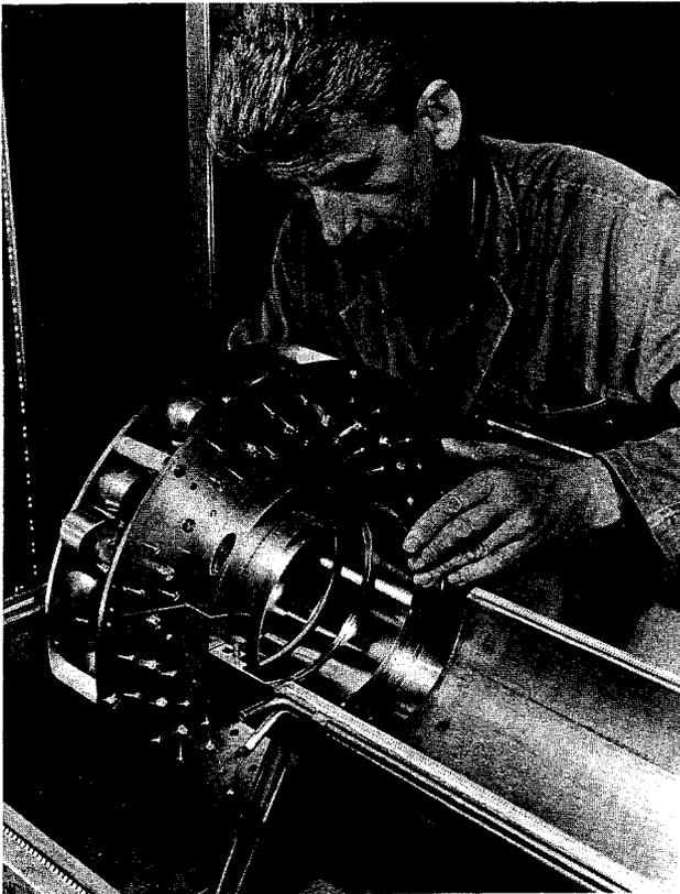
Fig. 4. Inside of an RF cavity.
