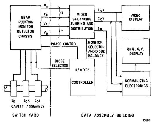
Fig. 4--Switchyard beam position monitor system
