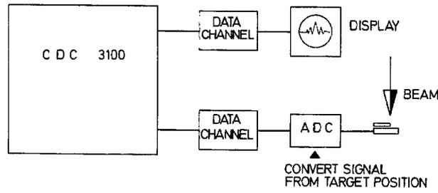
Fig. 2. Schematic of data transfer to and from the computer.
