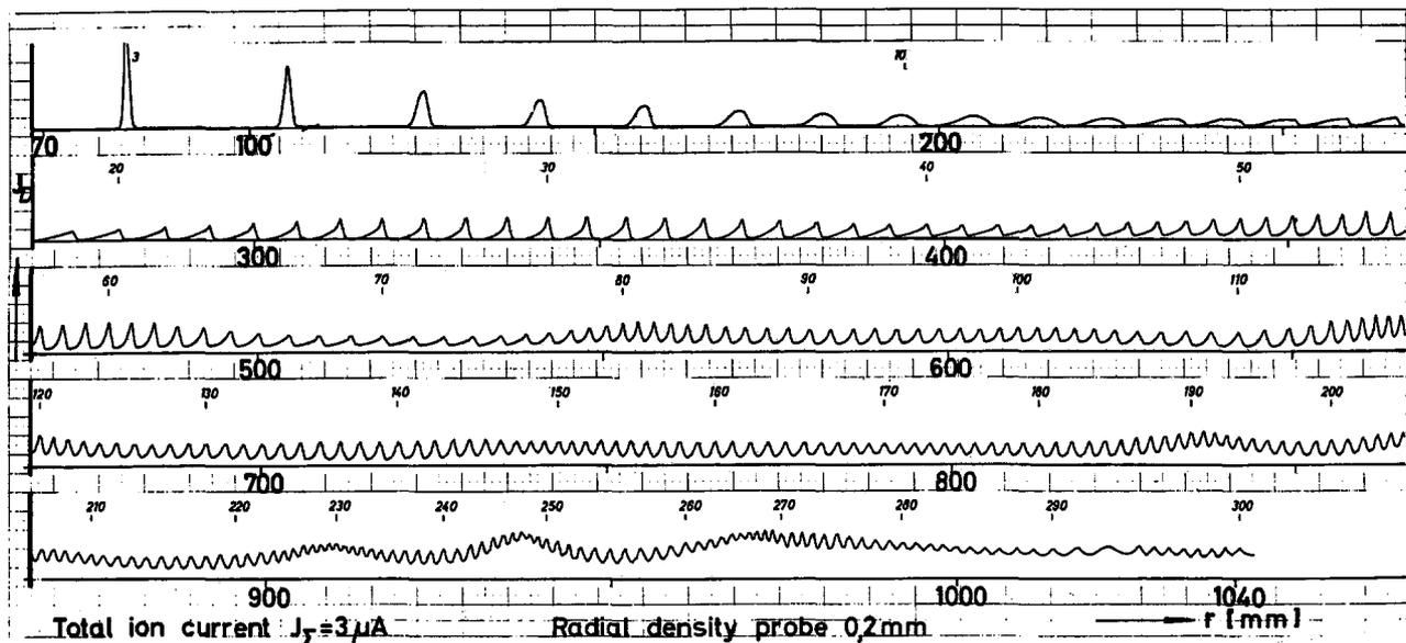
Fig. 1. Radial beam density in the Karlsruhe Isochronous Cyclotron. Large numbers below trace indicate the radius in mm, small numbers above give the turn number counted from machine center. Measurement was made with a Siemens Oscillomink recorder of 800 Hz nominal bandwidth.
