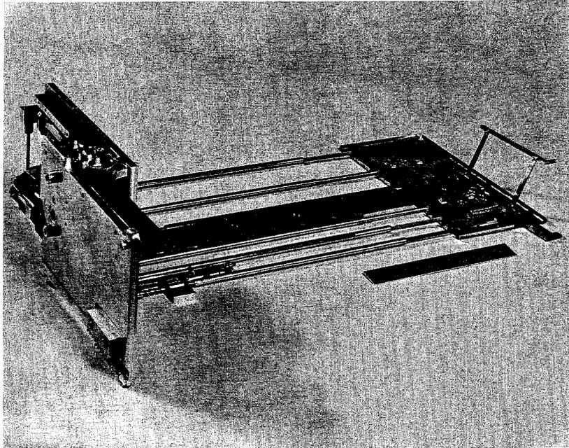
Figure 3 Mark IV Target Manipulator
