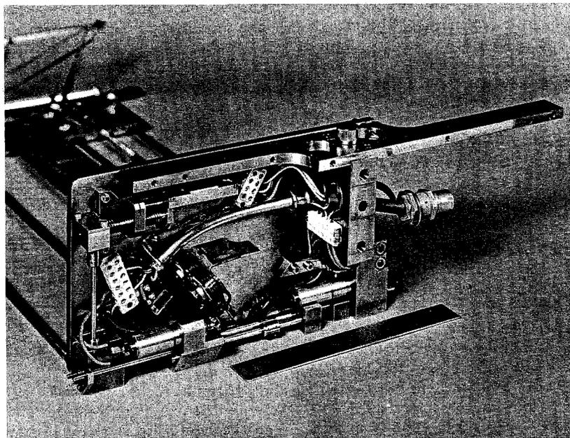
Figure 4 Drive Unit of Mark IV Target Manipulator
