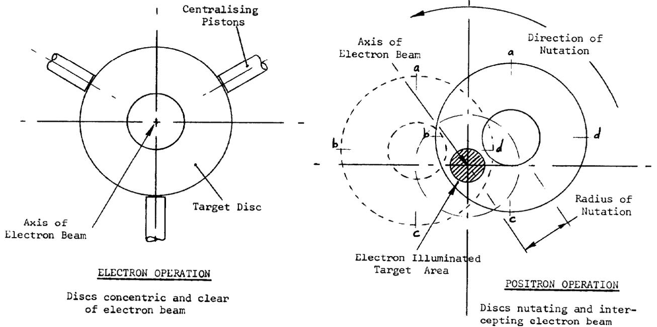
Fig. 1. Target Disc Positions.
