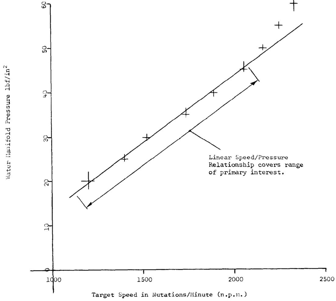
Fig. 4. Target Speed Graph.
