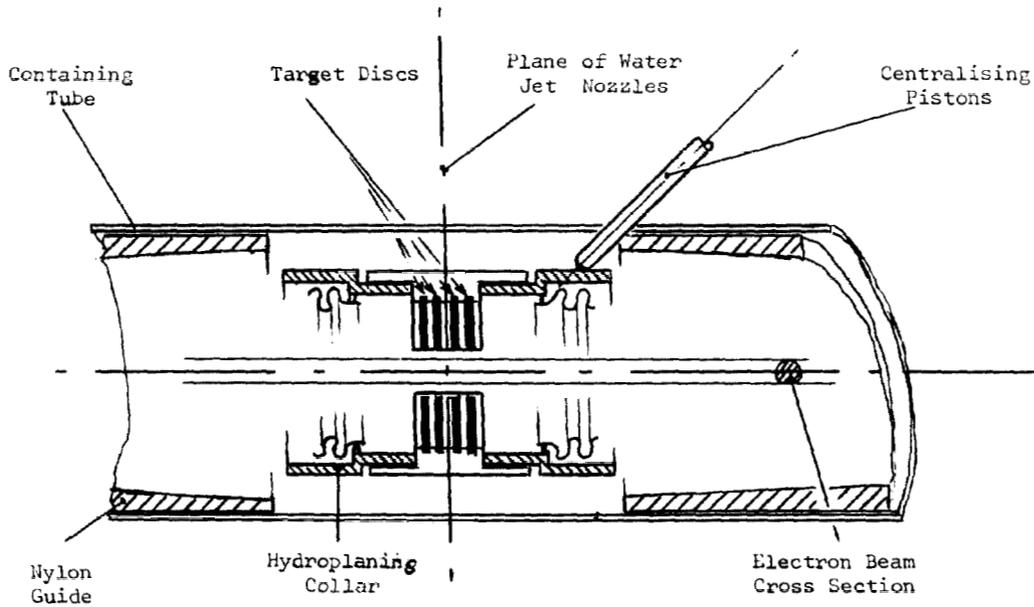
Fig. 6. Section of Target Capsule (Static).
