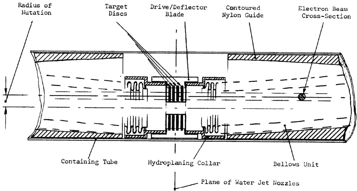
Fig. 2. Section of Target Capsule (Nutating).
