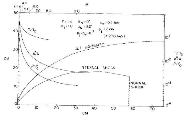
Fig. 3. Flow field for a freely expanding jet from a sonic nozzle ( $M_j = 1.0$ ) of 2 cm. diameter ( $\phi_j = 2$  cm) and a pressure ratio,  $p_j/p_\infty$ , of  $10^3$ . The left hand scale refers to the flow field boundary dimensions; the right hand scale to the gas properties normalized to the values at the nozzle. The required ion beam energy is  $\sim 230$  kev.
