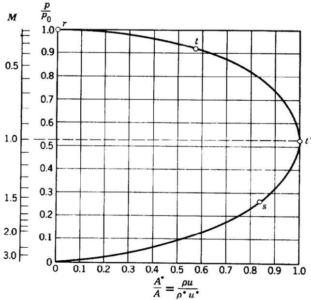
Fig. 1. Velocity as a function of normalized nozzle area for isentropic flow in the one-dimensional approximation. The flow in the expanding region of the nozzle is described by the lower half of the curve if sonic conditions are reached in the throat. (Ref. 2.).
