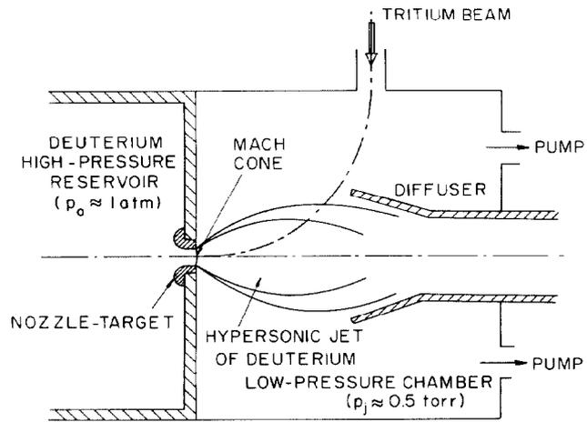
Fig. 5. Highly schematized configuration of a free-jet target. For the conditions used in computing Fig. 3 the nozzle to diffuser distance  $\sim 50 \text{ cm}$ , and the diameter of the low pressure chamber  $\sim 100 \text{ cm}$ .
