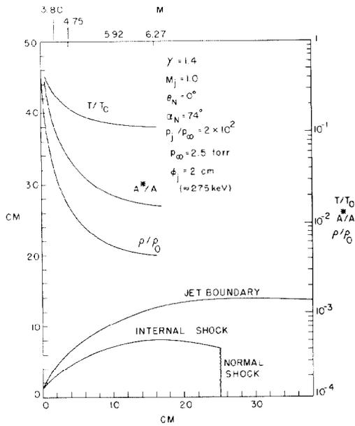
Fig. 4. The flow field for a pressure ratio,  $p_j/p_0$ , of  $2 \times 10^2$ . Note that the beam energy in this case is  $\sim 275 \text{ keV}$ .
