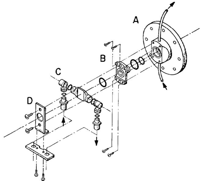
Fig. 1. Exploded View of Target Assembly
