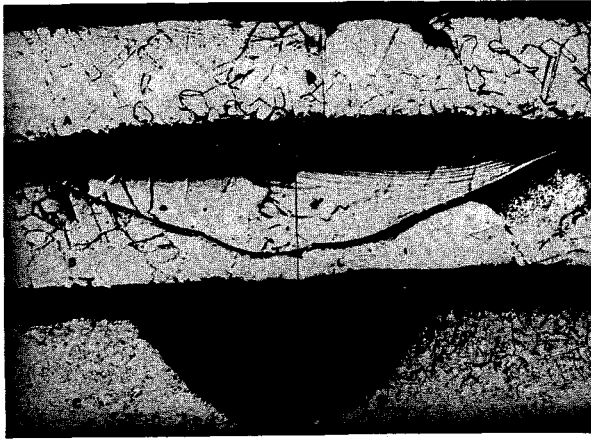
Figure 2. Transverse Cross Sections of Cu Target Backings Showing Modes of Failure. a./ Fissures in impure copper. b./ Partial melting in OFHC copper. c./ Puncture by melting.
