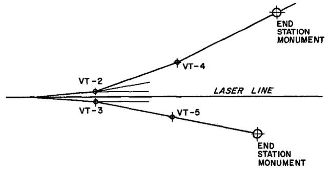
Fig. 6. Stretched wire layout for alignment of beam switchyard area.
