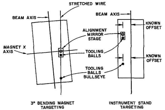
Fig. 8. Targeting on beam switchyard components.
