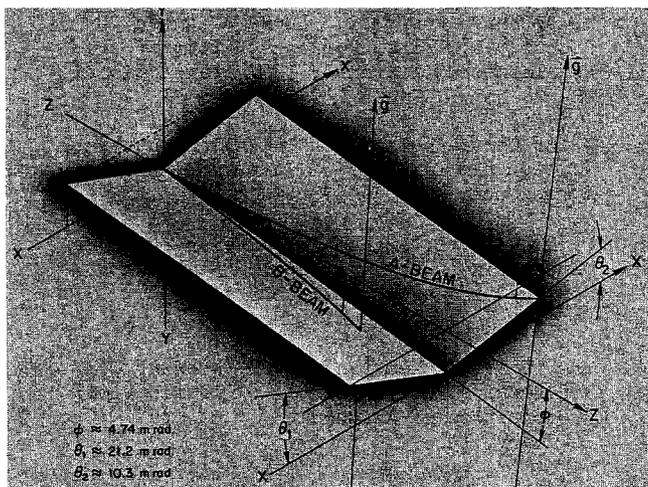
Fig. 3. Tilted planes of A and B Beams in the beam switchyard.
