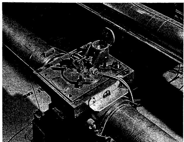
Fig. 4. Alignment equipment on laser target stand.
