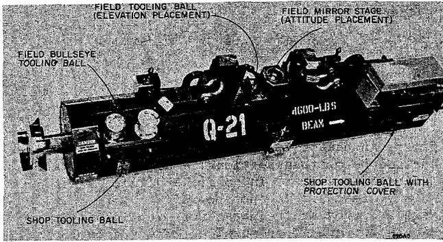
Fig. 5. Alignment equipment on a quadrupole magnet.
