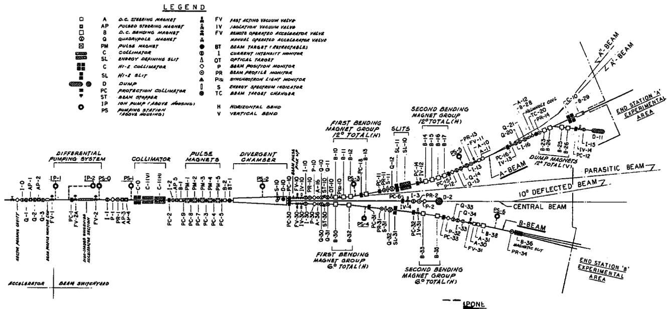
Fig. 1. Component layout of the beam switchyard for the two-mile linear accelerator.
