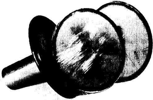
Fig. 13. View of edge weld and burr on cut open flanges.
