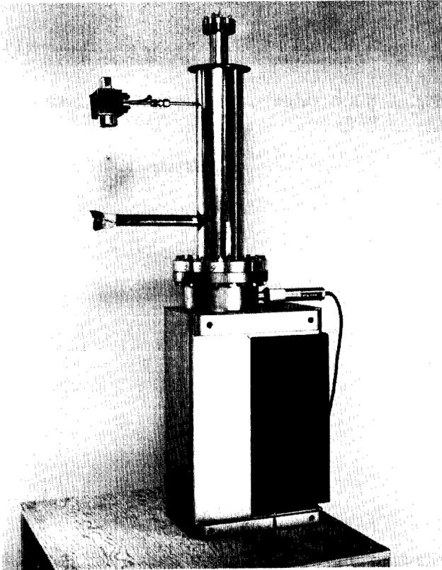
Fig. 1. Varian sputter ion pump, 140 l/s, with std. 4-in diam  $\times$  17-in s.s. tube.
