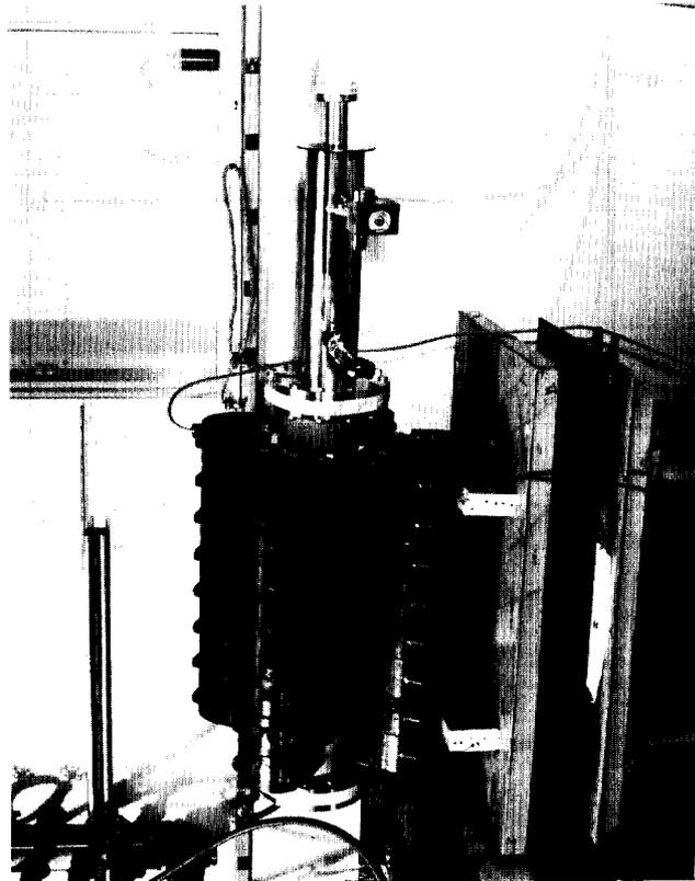
Fig. 2. R.C.A. sputter ion pump, 500 l/s, with std. tube.
