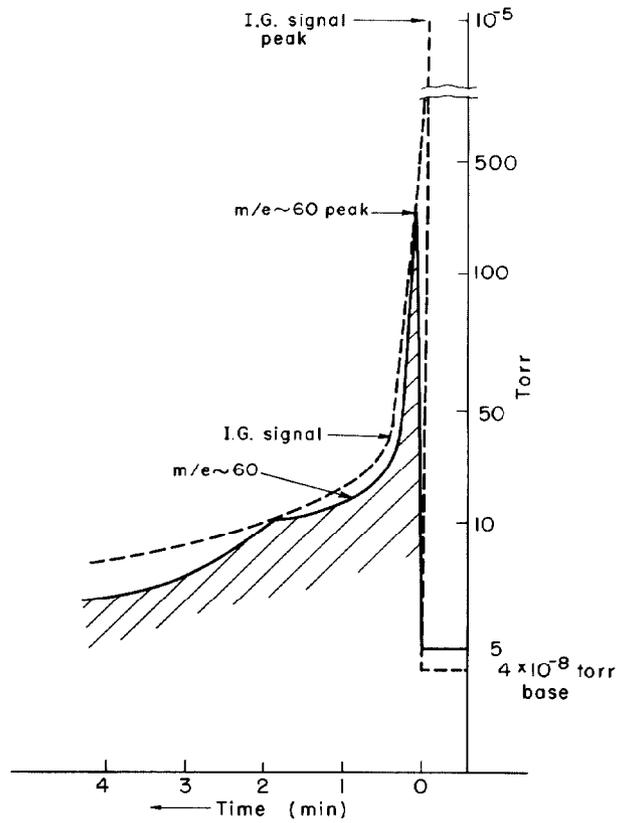
Fig. 7. Plot of single peak and BAG response to 200  $\mu$  gas pulse in foreline of Welch turbomolecular pump.
