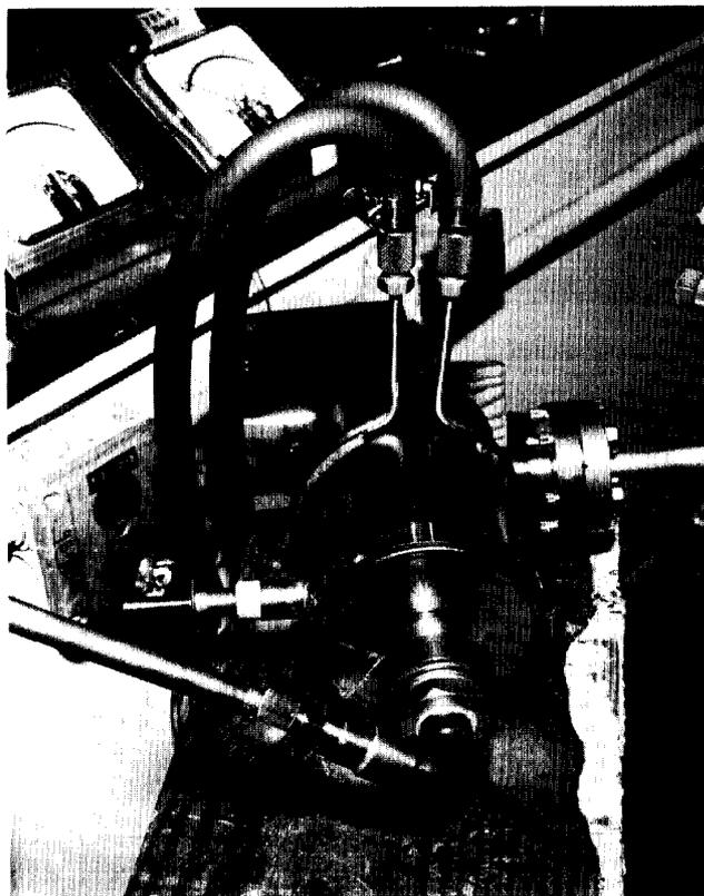
Fig. 9. Porous metal filter foreline trap and valve combination. Note electrode for  $^{12}\text{R}$  heating porous metal directly.
