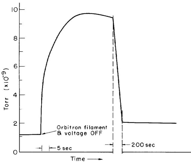
Fig. 8. BAG response vs time upon cutting off power to Orb-ion pump.
