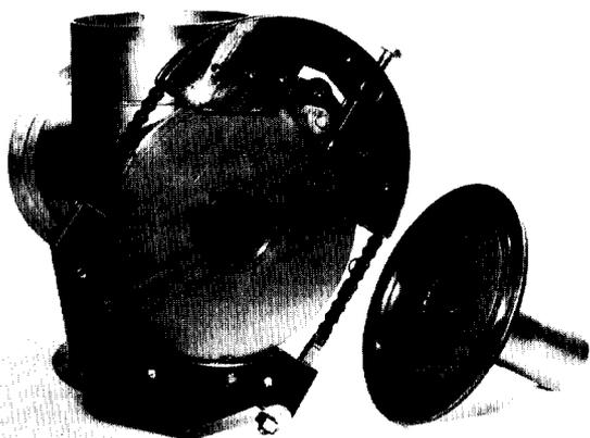
Fig. 11. Tool for cutting open edge welded flanges.
