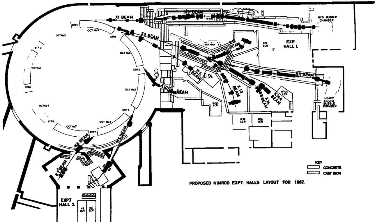
Fig. 2. The beam layout in the Nimrod experimental halls in 1967. X1 is an extracted beam feeding a target in for K9. X2 is a second extracted beam. K12 and K13 are beams at 15° production from the target. K11, K14 and K14A are zero angle production beams.  $\pi$ 4, K10S,  $\pi$ 5 and K8 with K7' are internally derived beams.
