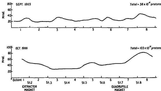
Fig. 1. Total integrated dose received by the Nimrod inner vacuum vessel up to October 1966.
