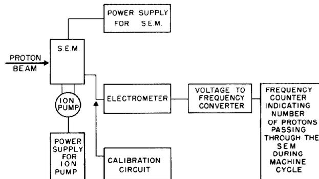
Figure 3 Schematic Diagram of Secondary Emission Monitor System
