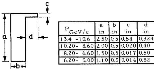
Figure 2 Plan View of Extraction Targets (All targets were 1/8-in in vertical extent)
