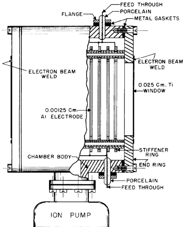
Figure 4 Secondary Emission Chamber and Vacuum Pump
