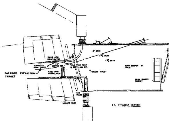
Figure 1 Targeting Straight Section Showing Parasite Extraction Target Position for Proton Beam Extraction and for Secondary Beam Down  $17\text{-}3/4^\circ$  Channel.
