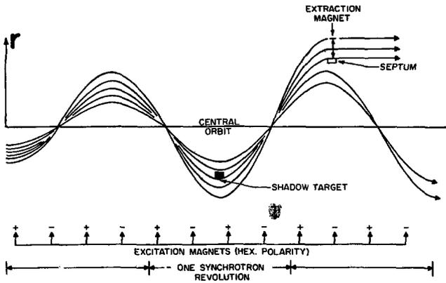
Fig. 3. Plot of particle trajectories with respect to central orbit followed 3 turns around the synchrotron. The location of the shadow target, the extraction magnet and septum and the excitation magnets are shown. The polarity of the hexapole field component is shown.
