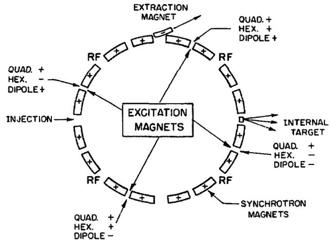
Fig. 2. Plan view of the synchrotron showing location of system components and polarity of fields used.
