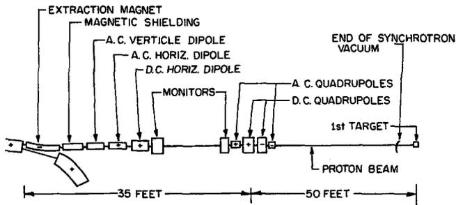
Fig. 5. Plan view of the external beam line to the first target. The various magnets and monitor boxes are shown.
