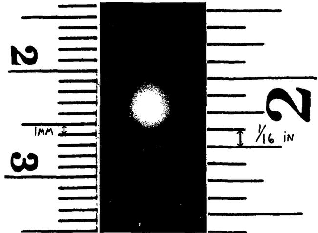
Fig. 6. Radioautograph made from a 0.010 inch Cu. foil placed at the first target point. Target exposure time 10 minutes at fixed momentum.
