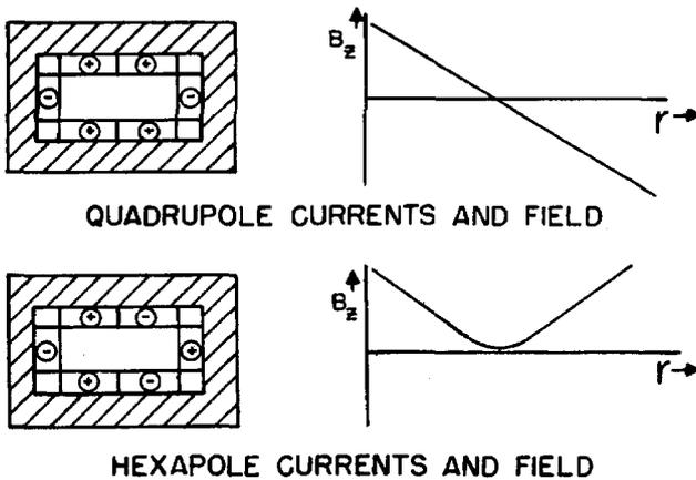
Fig. 1. Section through an excitation magnet showing directions of current flow and resultant fields on the median plane. In actual use these currents are superposed to give a combined but separately controllable field.
