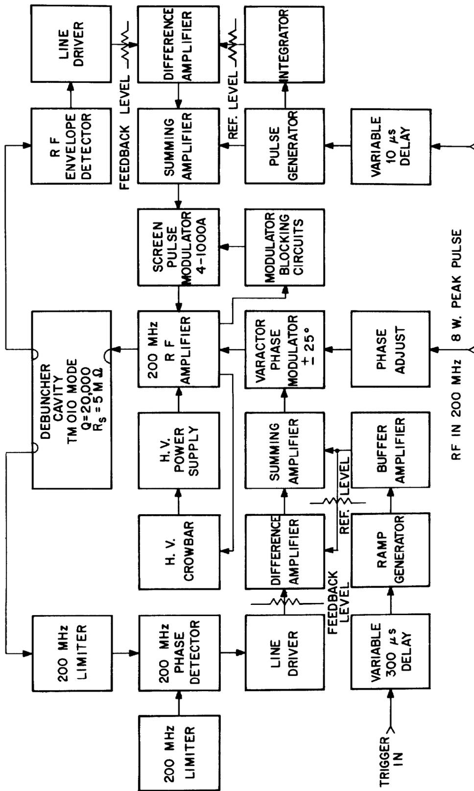
Fig. 3 Block Diagram of Variable Energy Debuncher RF System
