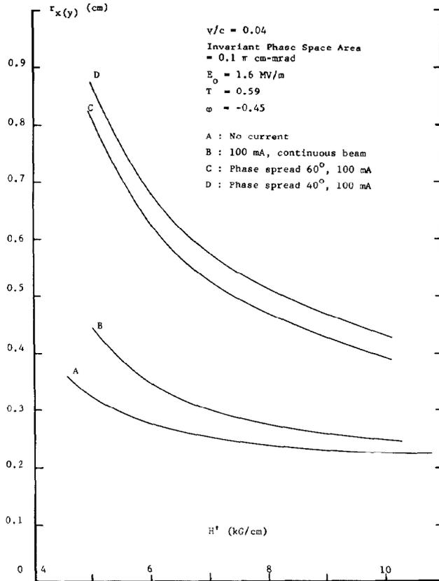
Fig. 5. Same as Fig. 4 for a higher current (100 mA) which corresponds to the new AGS injector linac at Brookhaven.
