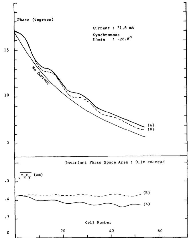
Fig. 6. Variations of the phase spread (half size) and  $\sqrt{r_x r_y}$  along the model linac cavity. For machine parameters, see Case (I) of Table 1. Curves (A) and (B) correspond to two different quadrupole strength distributions.
