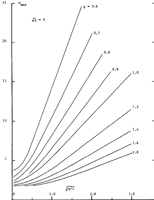
Fig. 1. Maximum betatron oscillation parameters  $w_{max}$  of (+)(-)(+)(-) quadrupole systems as a function of the space-charge parameter  $\sqrt{q/2}$  for  $\Omega = 0$  and  $g = 0.6 - 1.8$ . For definitions of  $g$ ,  $\Omega$ , and  $q$ , see Eqs. (14), (15), and (22), respectively. The maximum transverse size  $r_x$  (or  $r_y$ ) of the beam is  $w_{max} \sqrt{\lambda(\beta_S W)}$  where  $\beta_S W$  is the invariant phase space area.
