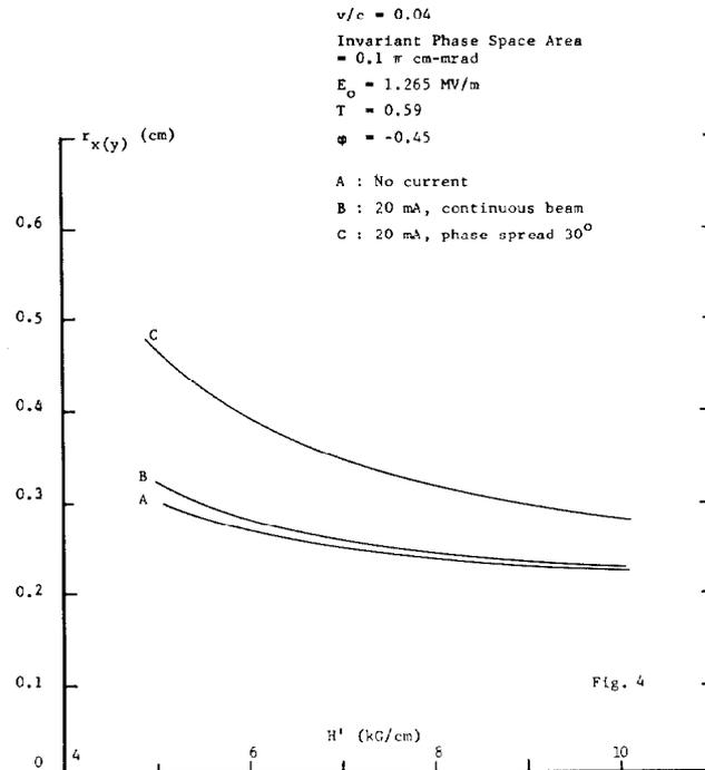
Fig. 4. Maximum transverse dimensions  $r_x$  (or  $r_y$ ) near the injection energy (0.75 MeV) as a function of  $H'$ , the quadrupole field gradient. Parameters are similar to those for the proposed Los Alamos linac.
