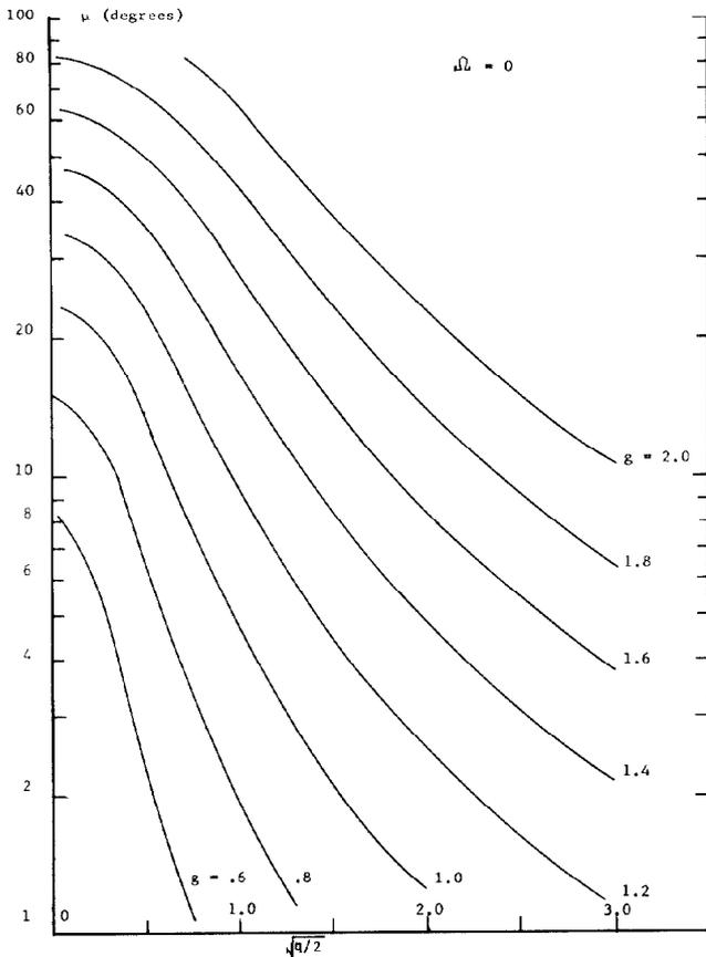
Fig. 3. The phase advance  $\mu$  (degrees) of the betatron oscillation per focusing period  $2\beta_S\lambda$  for  $\Omega = 0$  and  $g = 0.6 - 2.0$ . The wave number  $k_t$  of the transverse motion is  $k_t = (\mu/2\beta_S\lambda)$ .
