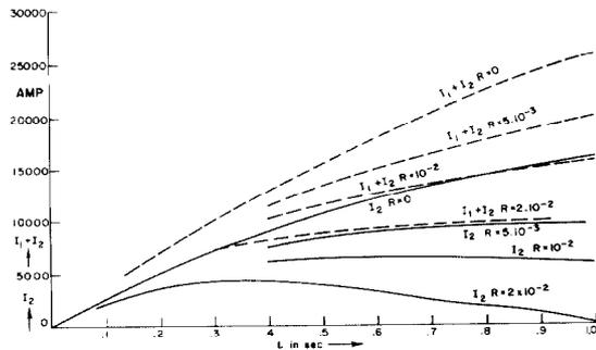
Fig. 3  $I_2(t)$  and  $(I_1 + I_2)(t)$  for Layer-to-Layer Faults during Rectification
