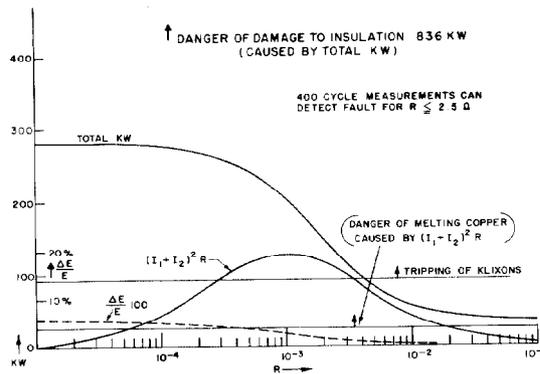
Fig. 8 Peak Power for Layer-to-Layer Faults
