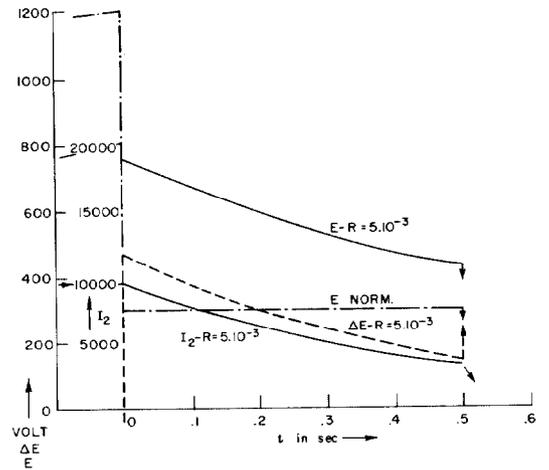
Fig. 7 Peak Power for Turn-to-Turn Faults
