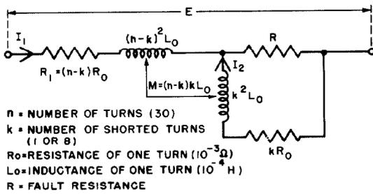
Fig. 1 Equivalent Circuit of Shorted Turn or Layer
