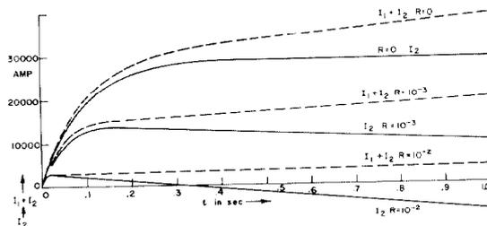
Fig. 2  $I_2(t)$  and  $(I_1 + I_2)(t)$  for Turn-to-Turn Fault during Rectification
