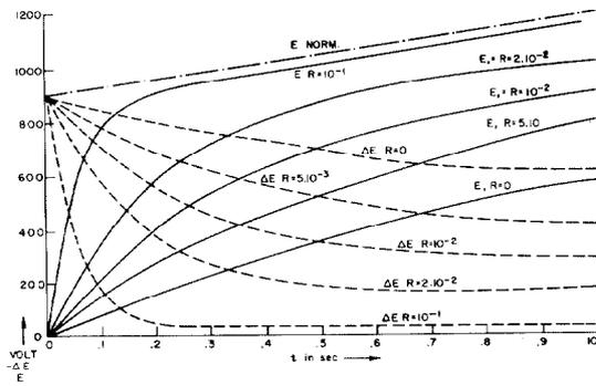
Fig. 6  $I_2(t)$  and Voltage E Across Faulted Octant for Layer-to-Layer Fault during Flat-Topping
