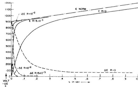
Fig. 4 Voltage E Across Faulted Coil for Turn-to-Turn Fault during Rectification
