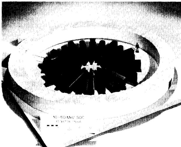
Fig. 1. Model of the 10-50-MeV SOC Showing Magnet Sectors Alternating with Accelerating Cavities. The beam is extracted at various energies with a moveable 90° magnet.
