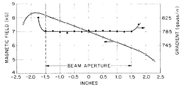
Fig. 6. Magnetic Field and Gradient vs Radius.
