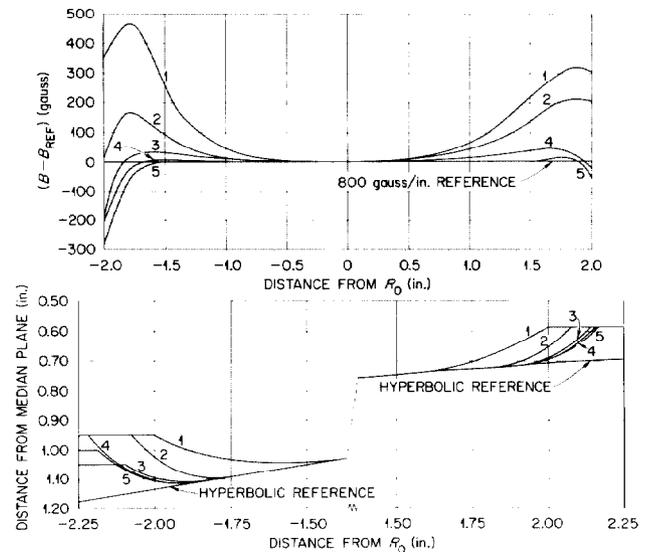
Fig. 5. Field Changes Produced by Changes in Pole Edge Geometry.
