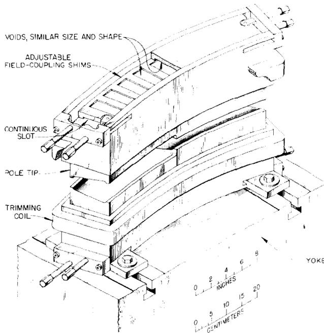
Fig. 4. A Pole-Tip Assembly Mounted on the Yoke.
