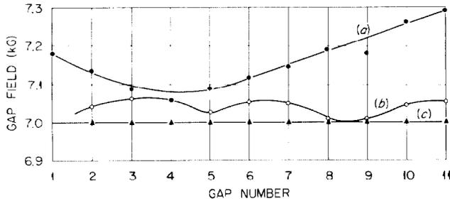
Fig. 7. Magnetic Field Measured at  $R_0$  for Each Gap (for reference only).
