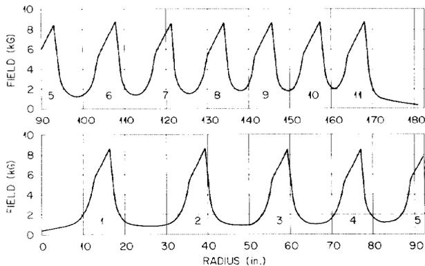
Fig. 8. Magnetic Field of the Prototype Sector with 11 Pairs of Pole Tips.
