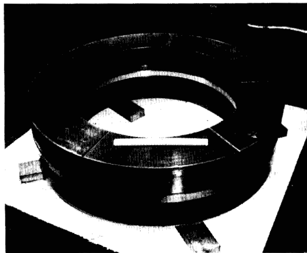
Fig. 6. Pole-tip ring assembled prior to being cut into six 60° sector magnets.
