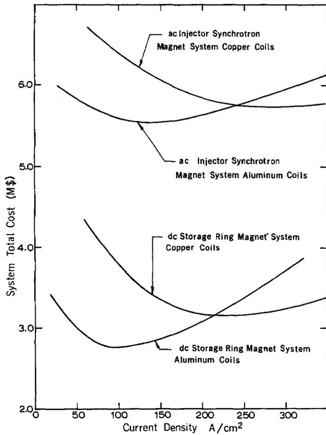
Fig. 5. Magnet system cost vs conductor current density.
