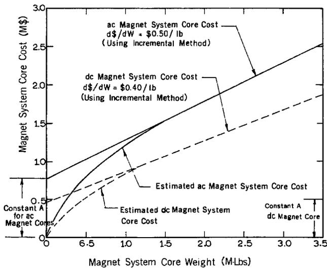
Fig. 3. Magnet core cost vs core weight, showing the derivation of the cost estimating equation for the core.
