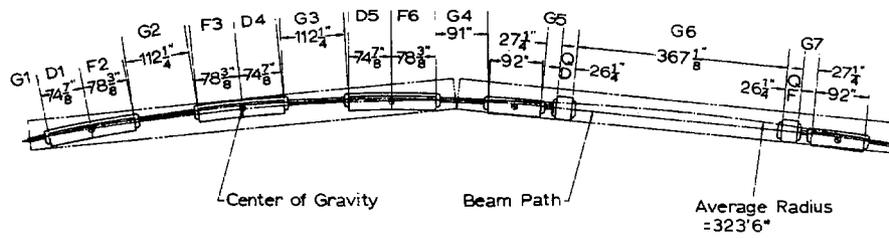
Fig. 2. A typical injector synchrotron superperiod showing the magnet elements, ac and dc.
