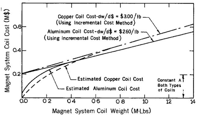
Fig. 4. Copper and aluminum coil cost vs coil weight showing the derivation of the cost estimating equation for the coils.
