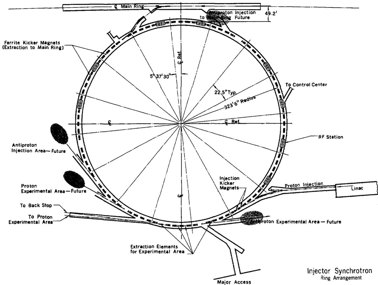
Fig. 1. Injector synchrotron ring arrangement.
