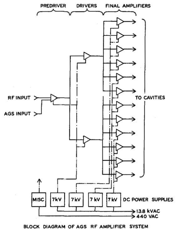
Fig. 2. Block diagram of AGS RF amplifier system.
