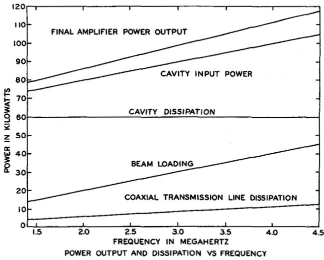
Fig. 1. Power output and dissipation vs. frequency.
