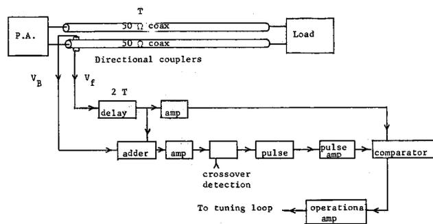
Fig. 4. Phase Detector.
