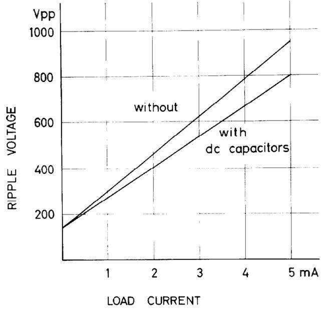
Fig. 2. Ripple voltage of the symmetrical 4 MV cascade generator with and without dc capacitors versus load current.
