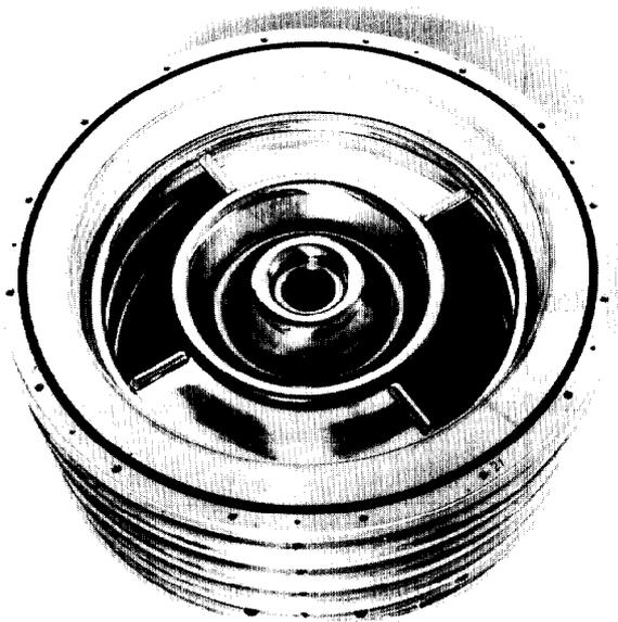
Fig. 5. Section of the 4 MV accelerating tube.
