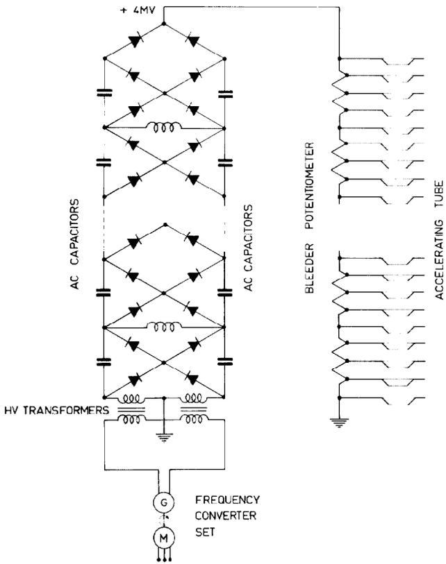
Fig. 1. Circuit diagram of the symmetrical 4 MV cascade generator.
