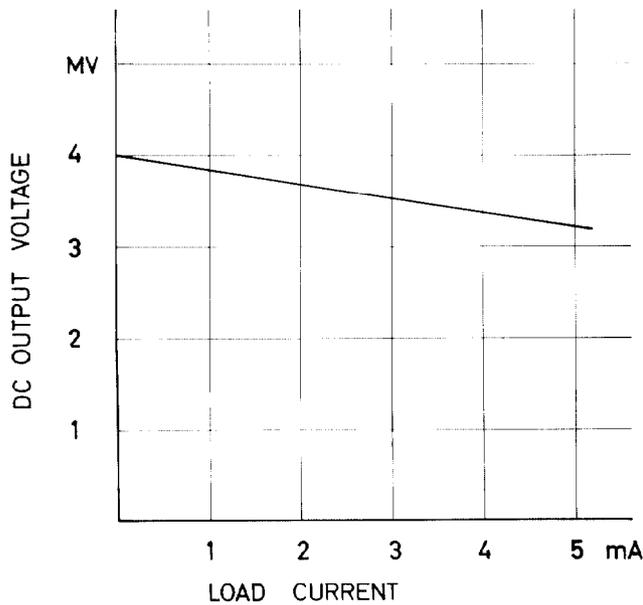
Fig. 3. DC output voltage of the symmetrical cascade generator at constant ac input voltage versus load current.
