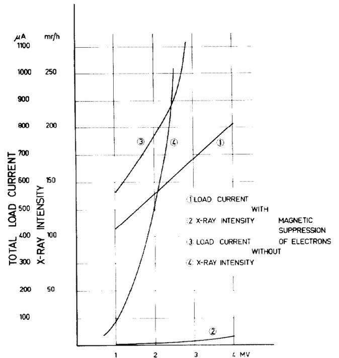
Fig. 8. Total generator load current and X-ray intensity with and without suppression of secondary electrons versus accelerating voltage.
