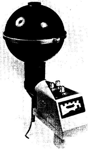
Fig. 4. Photograph of a muscle tissue equivalent ionization chamber survey meter.
