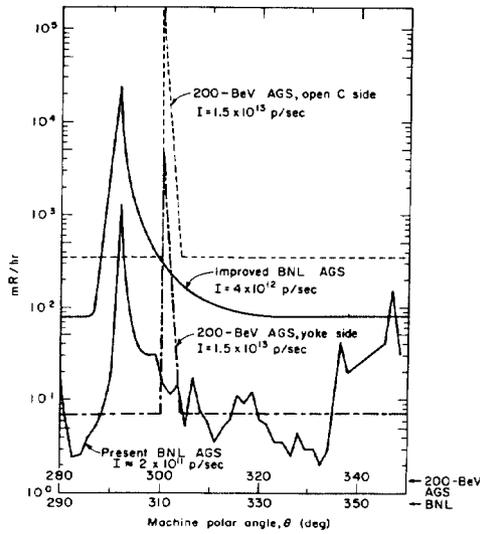
Fig. 1. Residual  $\gamma$ -fields at BNL and 200-BeV AGS vs machine polar angle. Measurements are taken between magnet ends, a few inches from vacuum chamber.
