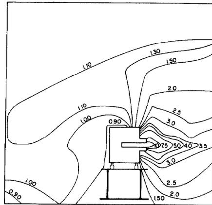
Fig. 2. Transverse  $\gamma$ -field at BNL-AGS magnet K8, 6 hr after machine turn-off.
