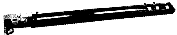
Fig. 4. Photograph of the coil system. On the right hand end the short coil is visible. On the handle of the coils, the mercury switch which was in series with the transistor switch is visible.
