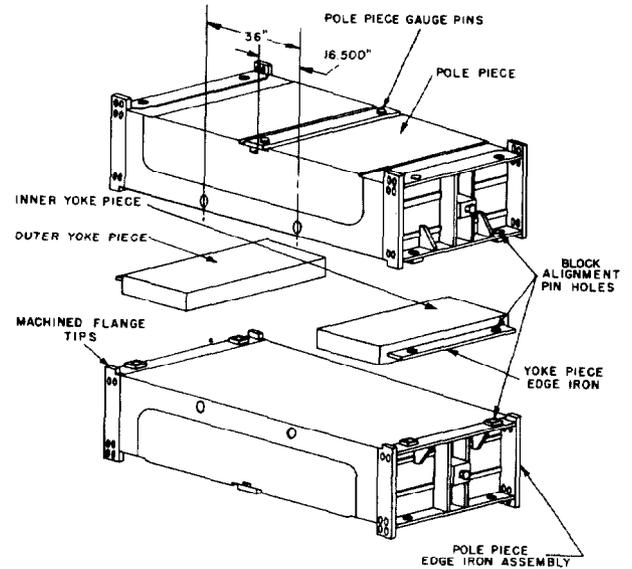
Fig. 5. Argonne ZGS Ring Magnet Center Block Assembly-Exploded View.
