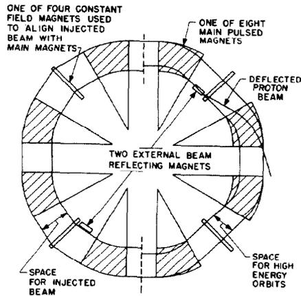
Fig. 2. Schematic of ZGS Magnet Plan.
