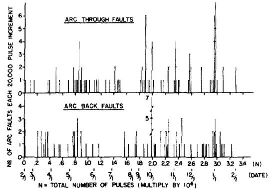
Fig. 7. Summary of Rectifier Faults.
