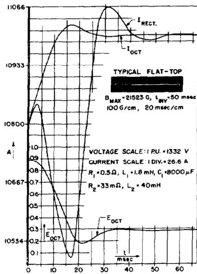
Fig. 5. Typical Transition into Flat-Top.
