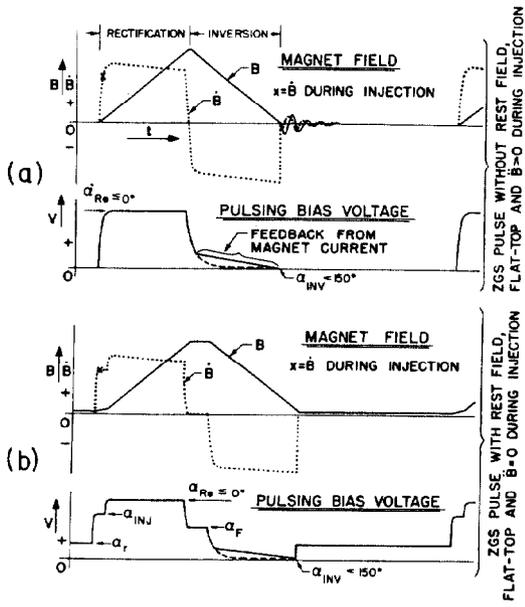
Fig. 2. Magnet Field and Pulsing Bias Voltage.
