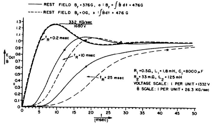
Fig. 4.  $\dot{B}$  at Injection.
