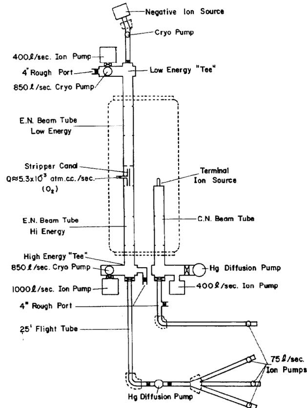
Fig. 1. A schematic diagram of the Tandem Accelerator showing the block diagram of the vacuum system. The C.N. portion of the accelerator was later removed.
