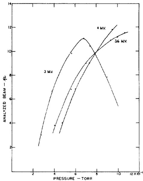
Fig. 6. Analyzed proton beam as a function of stripper gas pressure in the high energy beam tube for different terminal voltages. The injected beam was 30  $\mu$ a for all runs. The broken curves are incomplete because of high tube pressures.
