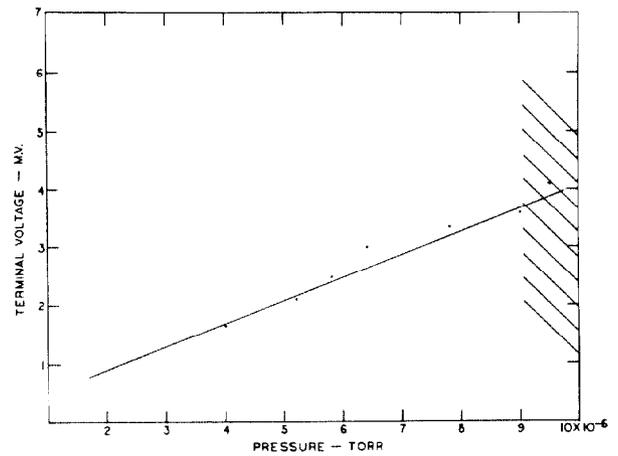
Fig. 5. The curve represents the maximum beam line at different terminal voltages with the corresponding stripper gas pressure in the beam tube. Voltage instability and eventual tube collapse is indicated by the hatched area.
