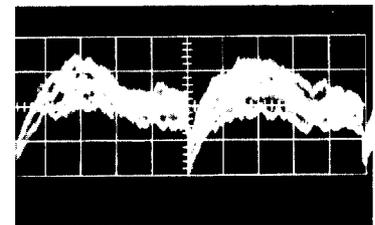
Fig. 2. Van de Graaf terminal voltage. Horizontal sweep: 10 msec per cm. Vertical deflection: 1.2 kV per cm.
