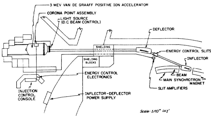
Fig. 1. Block diagram of Van de Graaf energy control system.
