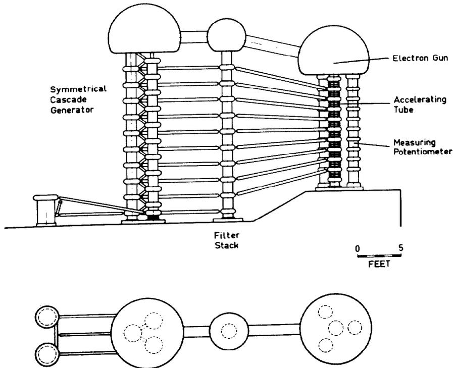
Fig. 2. Mechanical layout of the 1.5 electron accelerator.
