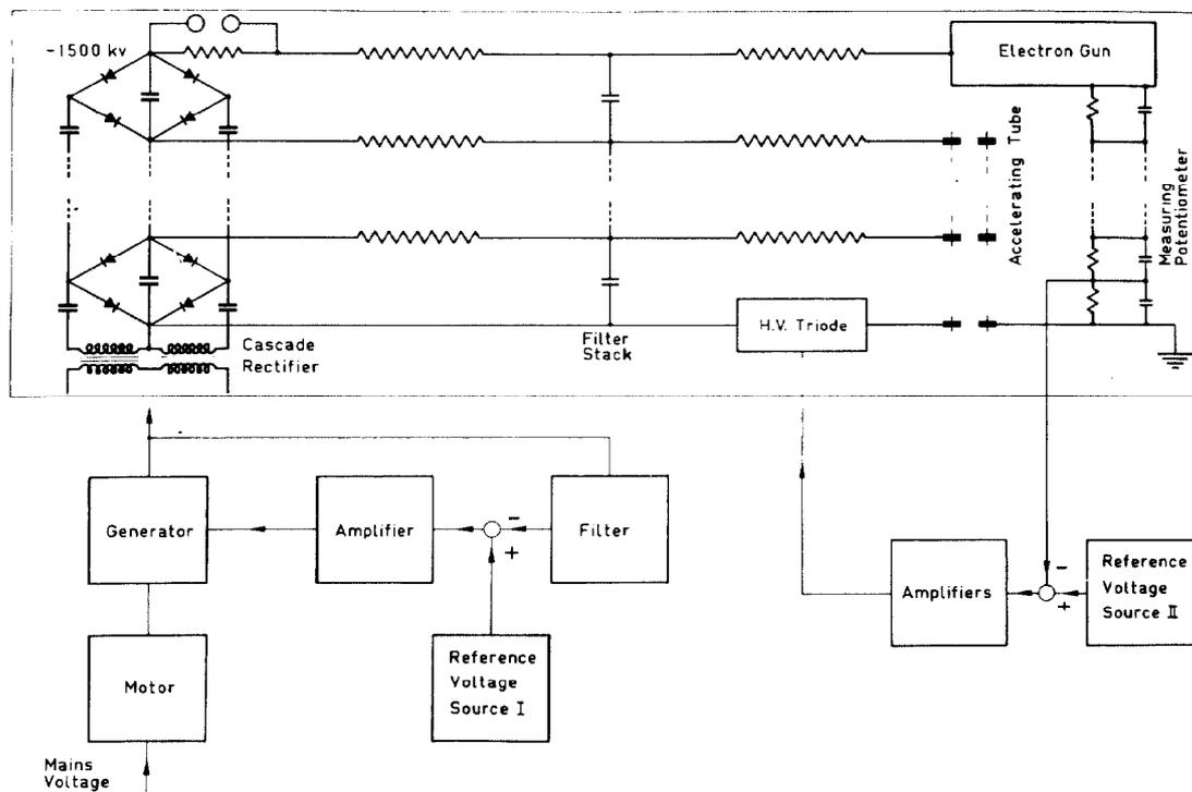
Fig. 1. Block diagram of the 1.5 electron accelerator.
