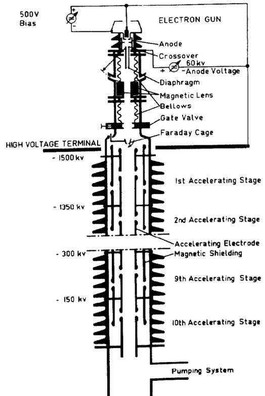
Fig. 4. Electron gun, injection system and accelerating tube of the 1.5 MeV electron accelerator.
