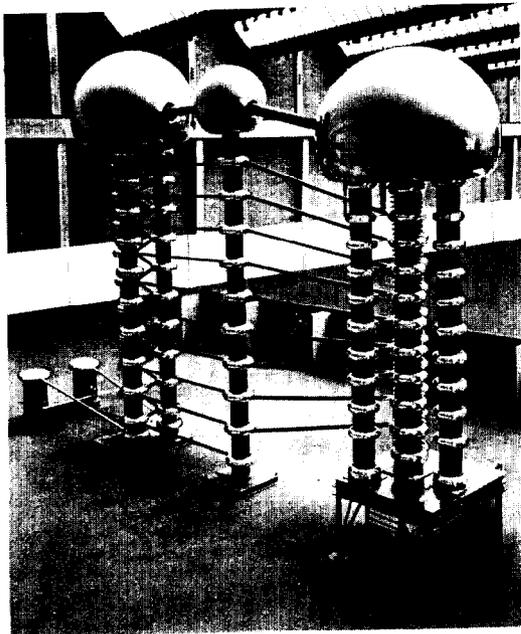
Fig. 3. 1.5 MeV electron accelerator during factory tests.
