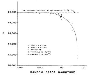
Fig. 8. Plot of computed Q as a function of random error magnitudes in a 165-cell tank with a Q ratio of 0.5 and h% bandwidth. The drive is in the center accelerating cell. Curves R2 and R3 variable are experimental; however, data points were too numerous for plotting.
