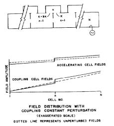
Fig. 6. Diagram showing result of coupling constant perturbation on field amplitudes. Note that there is no relative scale on these diagrams.
