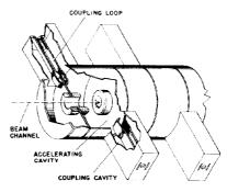
LOOP COUPLED ACCELERATOR STRUCTURE
