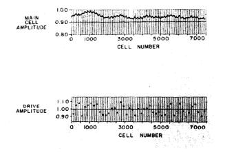
Fig. 13. Plot of accelerating cell and drive amplitude versus cell number for a case with R1 = 0.01%, R2 = 0.01%, R3 = 0.1%,  $Rh = 10^{\circ}$ , and R5 = 10.0%. The tank is the same as for Figs. 11 and 12.
