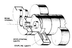
Fig. 3. Side-coupled structure with post-loaded resonant coupling cells.
