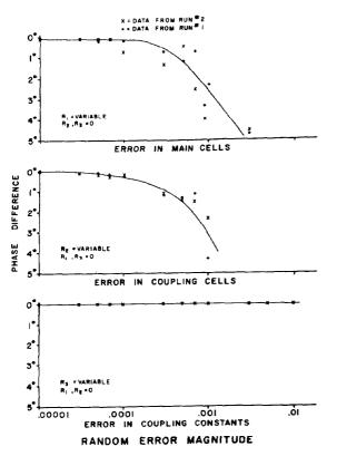
Fig. 10. Plot of computed phase differences as a function of random error magnitudes for the same cases as Figs. 8 and 9.
