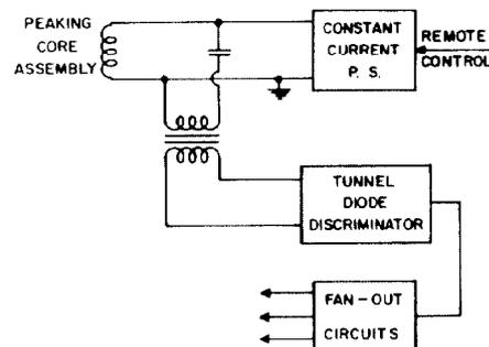
Fig. 2. Sketch of the electronics associated with the peaking cores. All the circuits use transistors except for the use of pass-tubes in the constant current power supplies.
