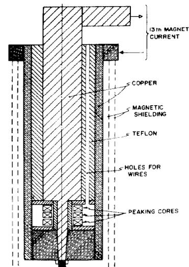
Fig. 1. This sketch shows the assembly for the peaking core. The coaxial current conductor was wrapped with a magnetic shield (conetic AA) and forcibly oil cooled.
