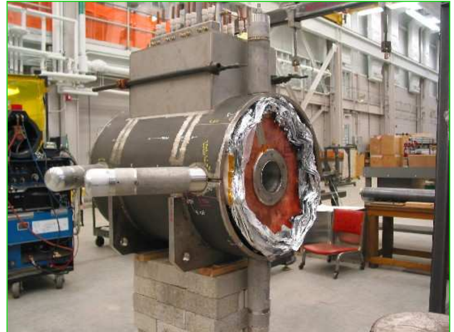
The SuSI magnet cryostat before the super insulation is applied to the front and back end of the liquid nitrogen thermal shield.
