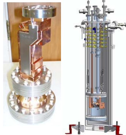
Figure 3: Picture of mushroom cavity attached to the mode launcher (left), and vertical cryostat (right).
