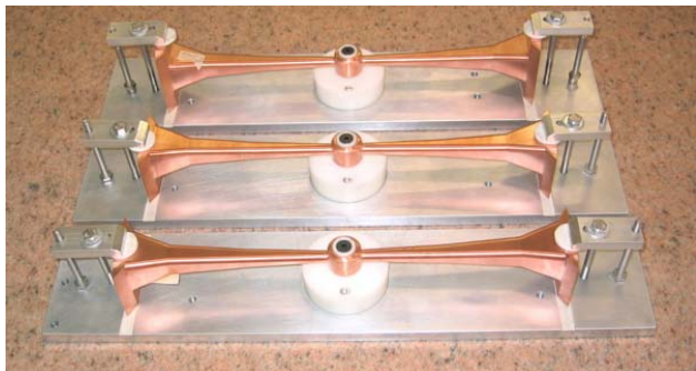
Fig. 1: The three OFE-Cu spokes finished and ready for assembly inside the resonator.
