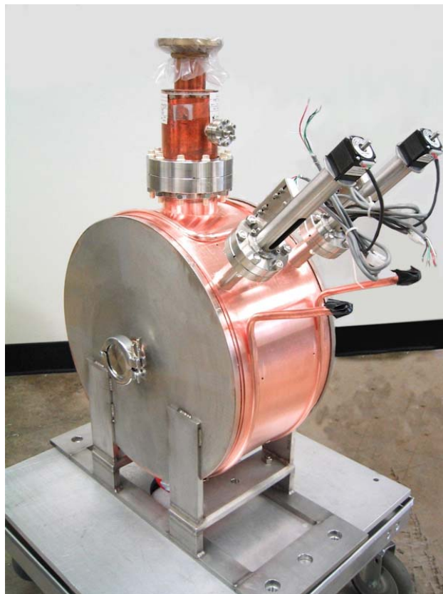
Fig. 3: The fully dressed prototype, the universal stand is visible at the bottom bolted to the resonator's support brackets. The same stand is used for all the resonators.
