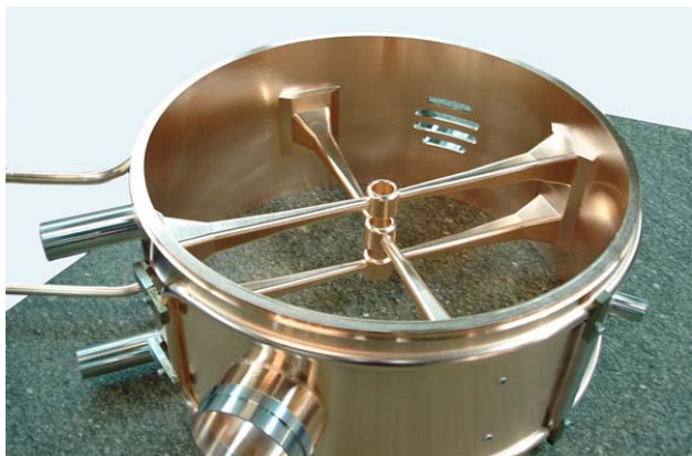
Fig. 2: The resonator after brazing of the spokes and ready for welding of the flanges. Two shoulder screws are visible on the bottom right.
