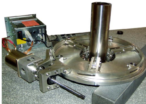
Figure 7: The first slow tuner prototype mounted on helium vessel end wall mockup. The stepping motor used in the tests is larger than planned for the cavity.
