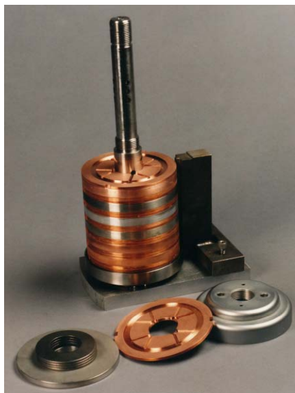
Figure 2c: The FNAL Pbar Target-Various materials 800 J/g pulsed air-cooled.
