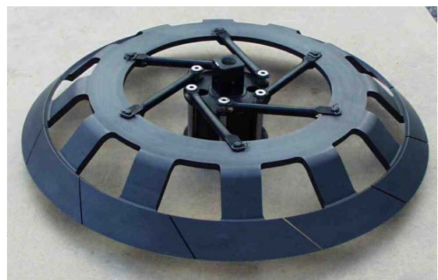
Figure 2b: The PSI Target-M – Carbon 30W/g CW radiation-cooled.
