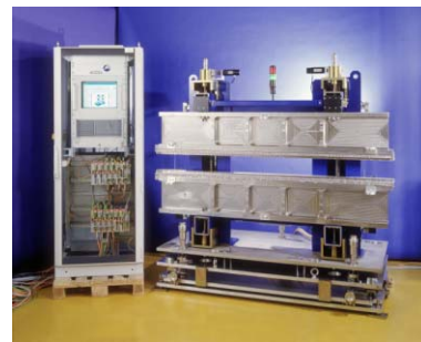
Figure 5: 6 identical PPM undulators for the SPARC project.
