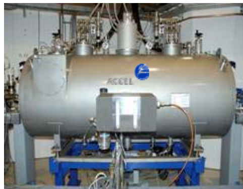
Figure 2: ANKA SCU installed into the storage ring.
