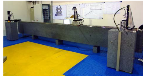
Figure 4: 7-m granite measurement bench equipped with a flip coil and a 3D hall probe.
